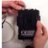
4. Connect the microphone cord to the LOUDMOUTH. Screw it down finger tight. Do not tighten with pliers.
